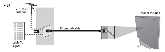
\* Once connections are completed, turn on the unit and begin initial setup. Channel scanning is necessary for the unitto memorize all available channels in your area. (Refer to "Initial Setup" on page 13.)
